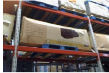
Oversize Packaging without proper reinforcement
